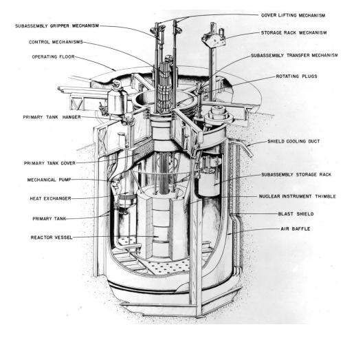
Figure 1-12. Cutaway View of EBR-II Pool-Type Primary System
