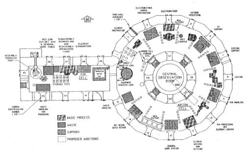
Figure 8-4. Air and argon cell proposed process equipment locations
