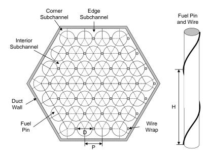
Figure 14-3. Fuel pin arrangement in a hexagonal duct
