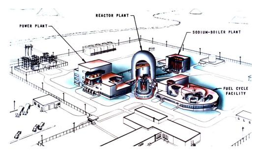
Figure 1-11. Rendering of the EBR-II Plant and its Fuel Cycle Facility
