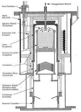
Figure 8-7. Schematic of Cathode Processor
