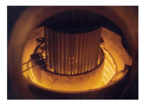
Figure 6-8. Injection-casting fabrication technique
