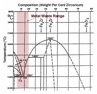
Figure 8-11. Iron-zirconium phase diagram [9]
