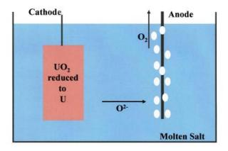
Figure 10-1. Electrolytic reduction process
