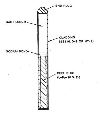
Figure 6-1. Schematic of metal fuel
