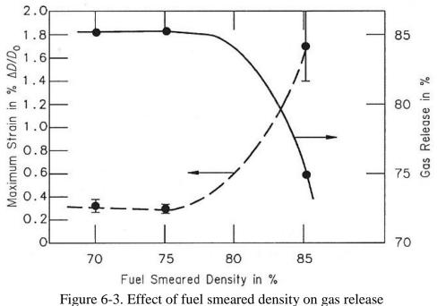
and cladding diametral strain
