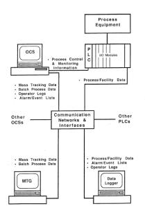
Figure 8-9. Process control and accountability system layout
