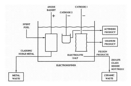
Figure 8-2. Schematic illustration of electrorefiner
