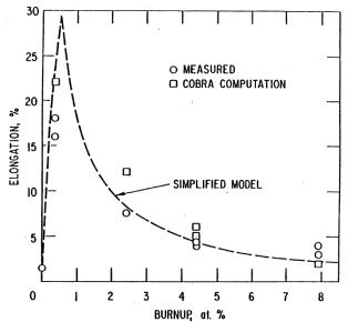
Figure 7-8. Pre-failure axial fuel extrusion as a function of burnup for metal fuel
