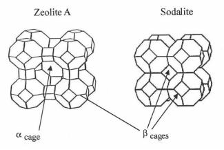
Figure 8-13 Molecular structure of zeolite and sodalite
