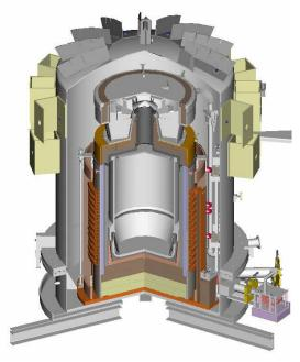
Figure 8-12. Metal Waste Form Furnace
