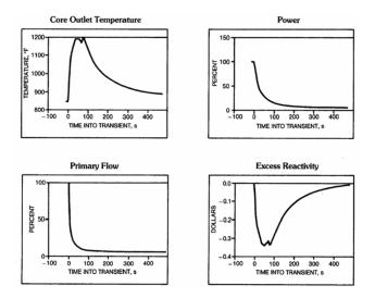
Figure 7-1. Unprotected loss-of-flow test results
