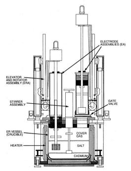
Figure 8-5. Schematic of electrorefiner
