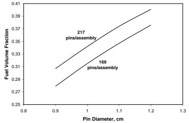
Figure 14-5. Comparison of fuel volume fraction as a function of pin diameter between 169 vs. 217 pins per assembly
