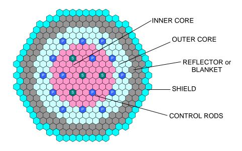
Figure 14-4. Typical hexagonal core layout
