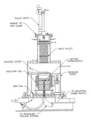
Figure 8-8. Schematic of injection casting furnace
