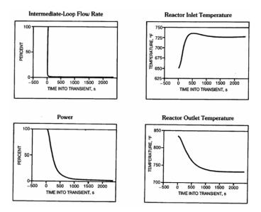
Figure 7-3. Unprotected loss-of-heat-sink test results
