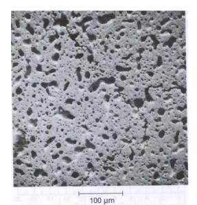
Figure 6-2. Fission gas pore structure of irradiated U-10Zr fuel
