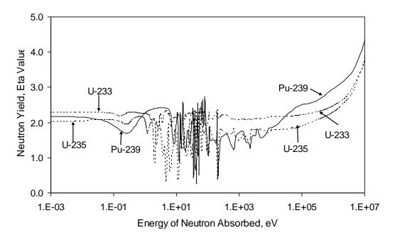
Figure 14-1. Neutron yield vs. neutron spectrum
