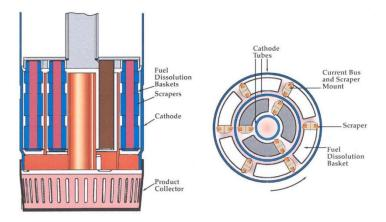
Figure 10-2. Schematic arrangement of Mark-V electrode
