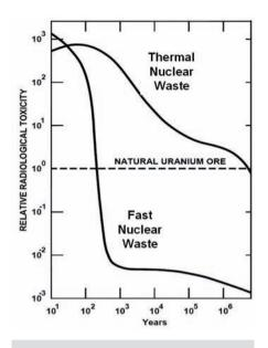
Figure 2: The fission products will only be radioactive beyond the level of natural ore for a few hundred years
