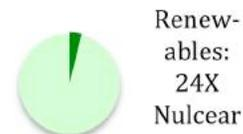
But since wind typically has one-third the capacity factor of nuclear, the actual steel-per-megawatt gap between the two technologies is more like 24X.
